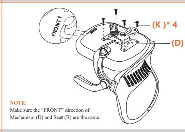
Using Wrench (O), attach Mechanism (D) to the Seat (B) with Bolts (K)\*4.
