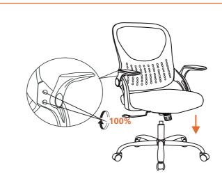
Using Wrench (O), 100% tighten the previously installed Bolts (N)\*4 on the Armrests (C)x1Lx1R. Align the hole on Mechanism (D) with Gas Lift (E), and press the Chair down until it is fully secured.
