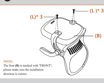
Turn the Seat (**B**) upside down . Using Wrench (**O**), install Armrests (**C**)x1Lx1R to the Seat with Bolts (**L**)\*6.
