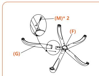
Turn the Base (F) upside down, insert the Legs (G)\*5 into the Base one by one. Use Wrench (O), secure both with Bolts (M)\*10.
