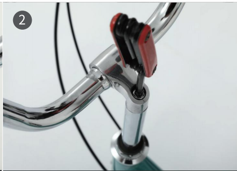
2. Tighten with a hexagon screwdriver.
