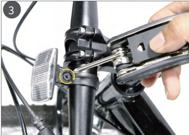
3. Use a screwdriver to install the front reflector near the center of the handlebar.
