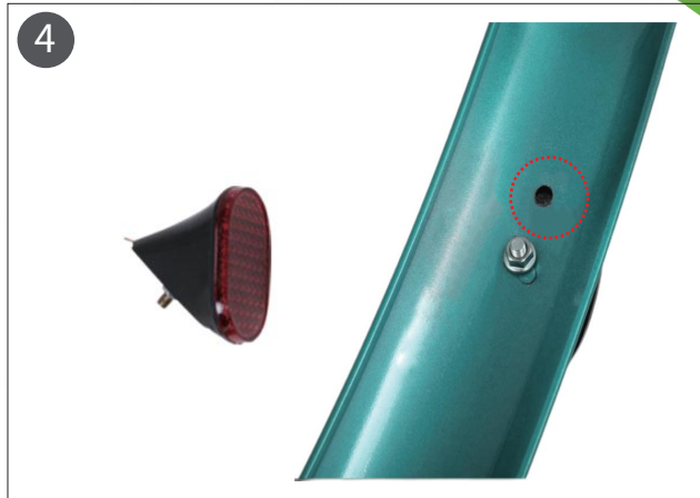
4. Position for installing the rear reflector
