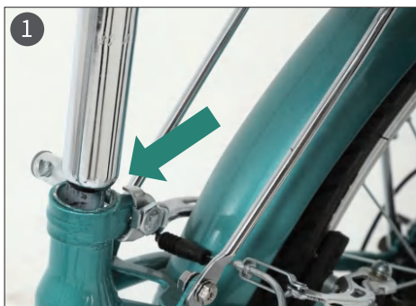
1. Insert the seat post into the frame.
