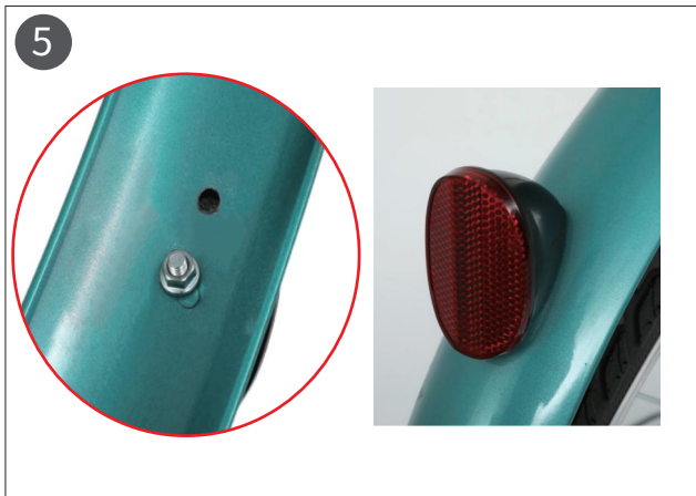
5. The rear reflector mounted on the rear fender
