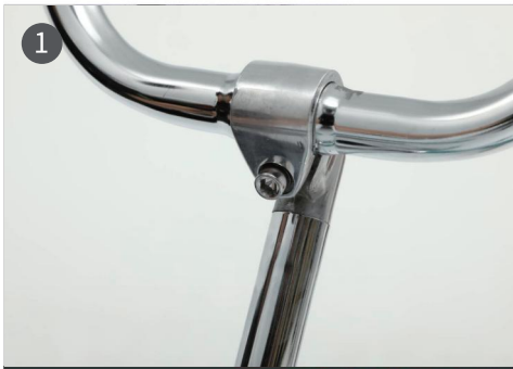
1. Insert the stem into the head tube.
