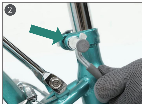
2. Tighten the seat post clamp.
