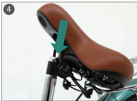
4. Insert the saddle post into the hole of the saddle.
