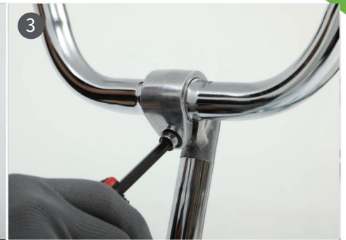
3. This screw controls the angle of the handlebar. Adjust the handlebar to parallel with the ground.
